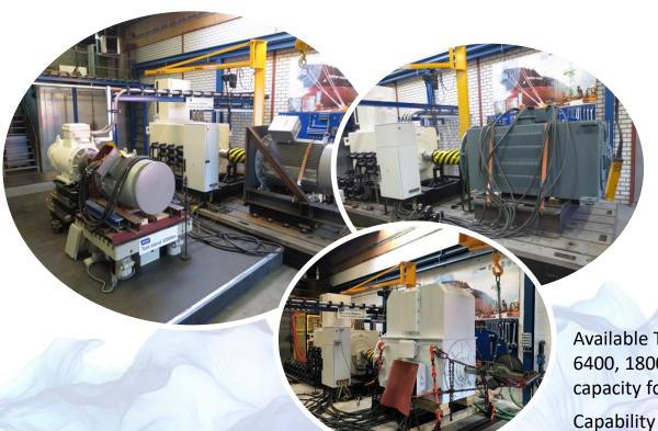
Full Load test up to 1 MW; 500-3600 rpm; up to 13.8kV
