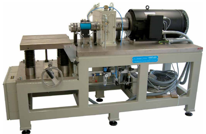
Electric motor test stand with lifting device and high-performance gearbox
