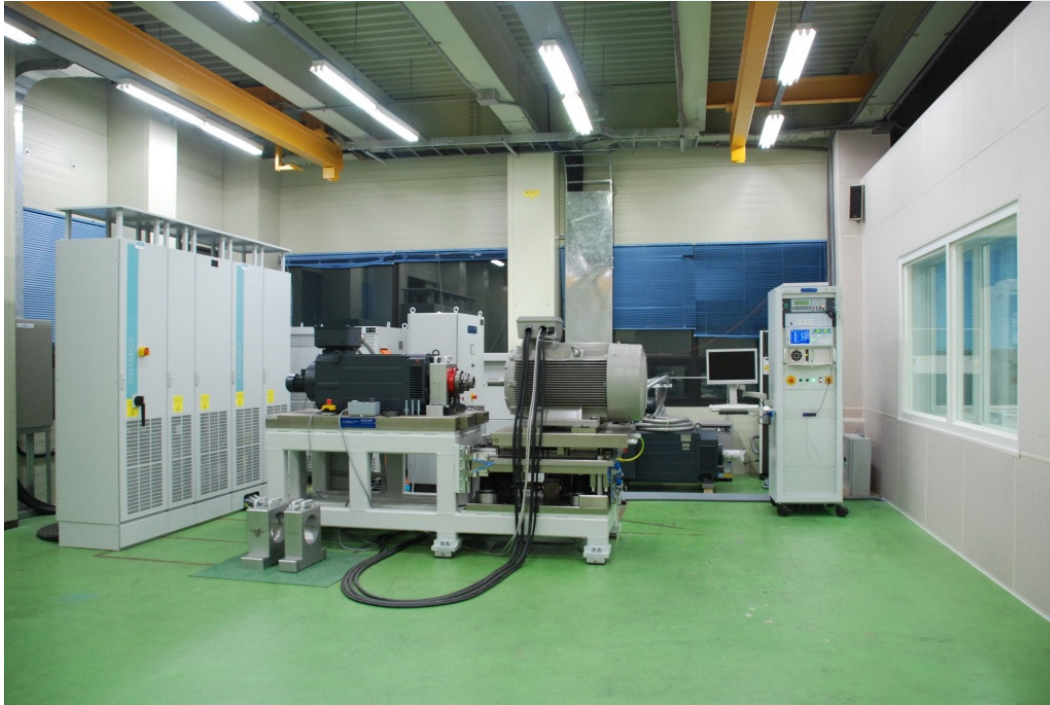
View of test stand#1 : largest dynamometer
