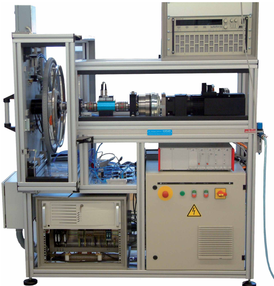
Test stand for wheelchair drives (Final inspection)
