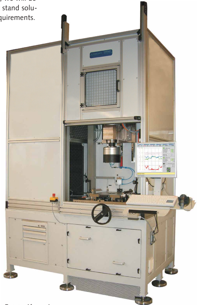
Test stand for gearboxes (Vertical measuring alignment)
