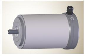
Triple protection against water penetration (slinger, long path, shaft seal from the inside) Quality ball bearings lubricated for life Conventional 6 pin Terminal Block
