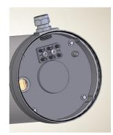
The motors are equipped with 3off drain holes which as standard come plugged with solid stainless steel screws. A capillary drain plug is supplied loose (can be found inside the terminal box in a plastic bag).
